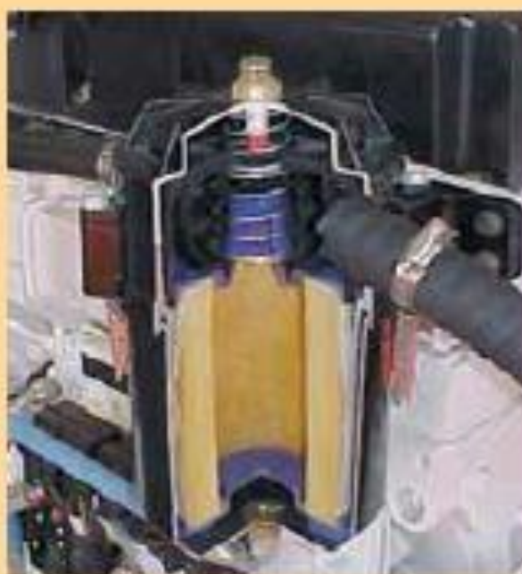
Cummins QSM11 marine engine with CCV cutaway
